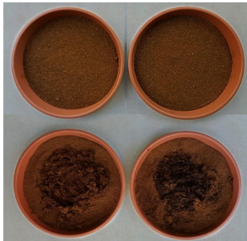
Plate 2: Samples of SpillFix before and 8 minutes after treatment with vinegar (left) and bleach (right).
